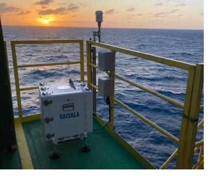
WindCube Offshore is a compact, lightweight and rugged remote sensing device. A highly refined, mature offshore technology, it provides unrivalled wind measurement capabilities and services for accurate, real-time 3D wind data.
