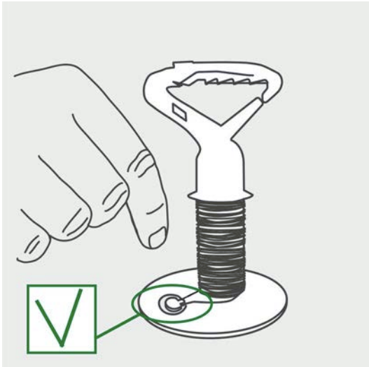
Figure 6 Unwinder Clip Is Level with the Unwinder Bottom Plate
