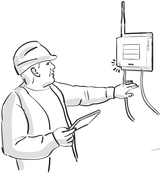
Install the access point requiring mains power and ethernet, or optionally a cellular modem
