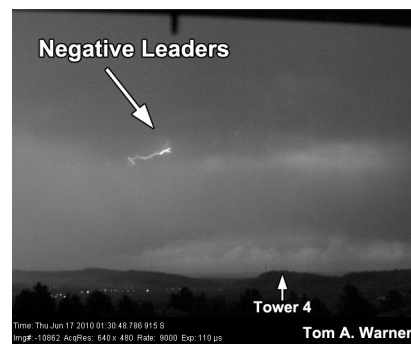
Figure 3. High-speed camera image (9,000 ips, 110 \mu s exposure) showing a NL propagating toward the towers following a +CG RS.
