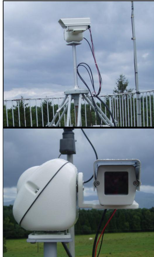
Figure 3. The Watec 902H camera with the pan/tilt uni, located in Lannemezan.
