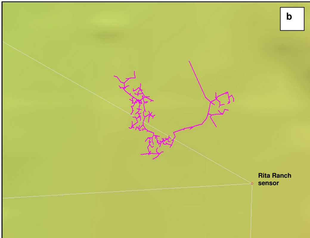
Figure 6: Close-up view of a large flash observed near the Rita Ranch sensor in the Tucson LS8000 network. (a) Individual VHF emissions located by the network. (b) after processing by flash algorithm.
