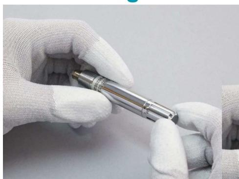
Use gloves (ESD gloves recommended) when attaching the sensor.
