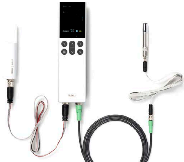
Indigo80 with GMP251 carbon dioxide probe and HMP110 humidity and temperature probe. The HMP110 probe offers measurement accuracy from ±1.0 °C and ±1.5 %RH (0–90 %RH) with higher accuracies available. The GMP251 CO 2 probe provides accuracy from ±0.1%CO 2 depending on operating conditions.
