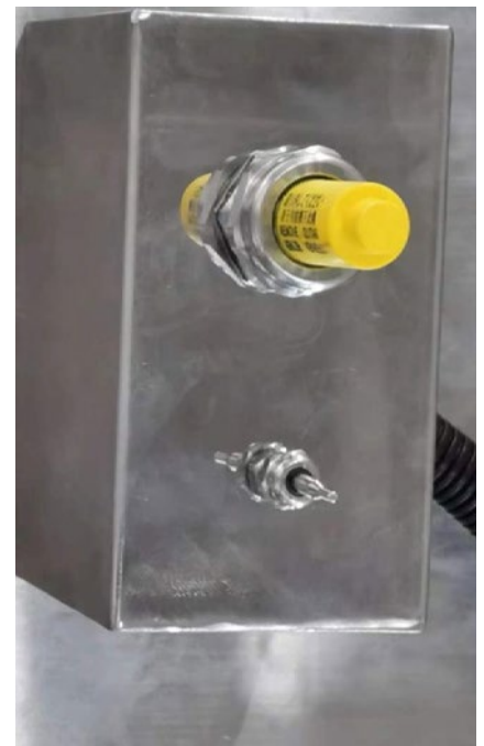
Installed HPP270 probes
